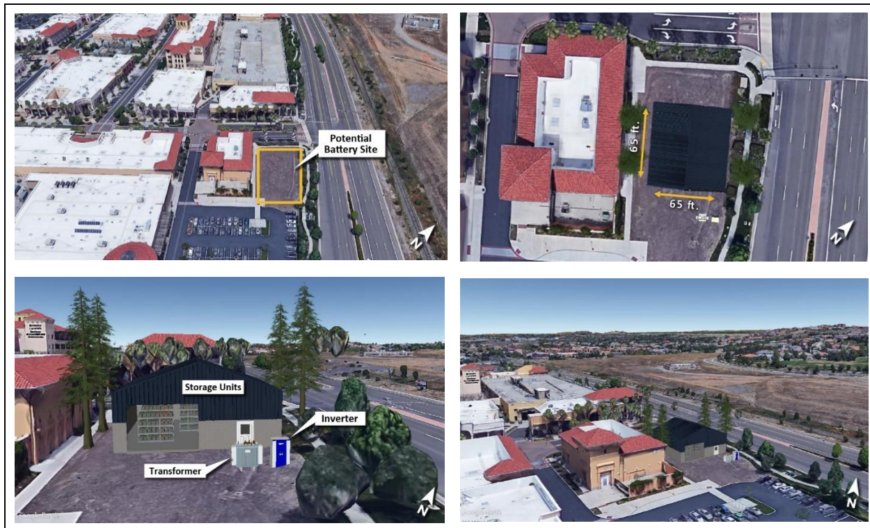
Figure 3-25. Example Energy Storage Facility Enclosed in Building
